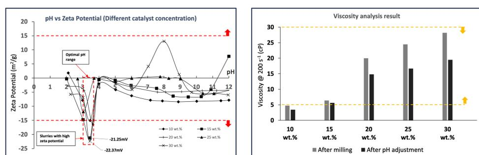
Fig. 2: Zeta potential (left) and viscosity (right) measurements of slurries with different catalyst concentrations
