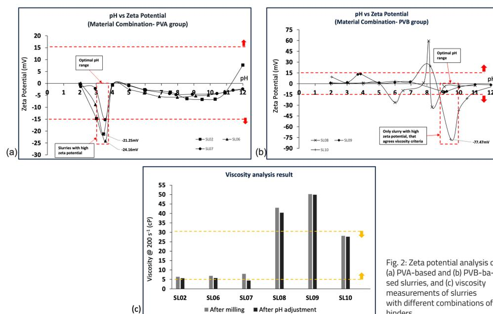
Fig. 2: Zeta potential analysis of (a) PVA-based and (b) PVB-based slurries, and (c) viscosity measurements of slurries with different combinations of binders
